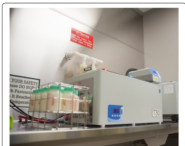
Figure 2 Pasteurization of donor milk. In North America, donor milk is pasteurized according to the Holder technique, which involves heating the milk to 62.5°C/144.5 °F and holding this for 30 minutes.
